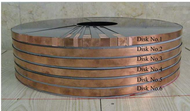
Fig. 1: Simplified transformer winding and disk numbering
