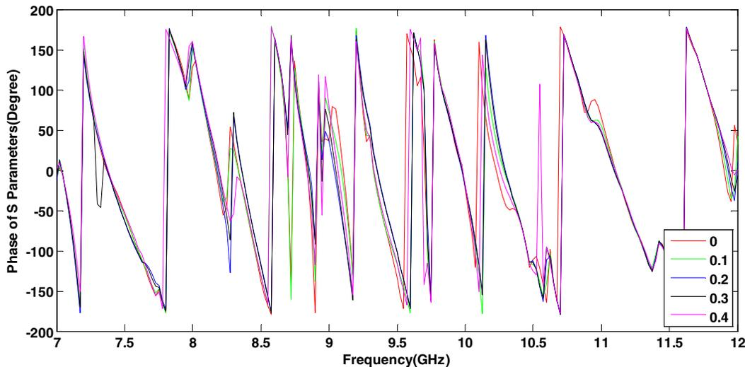
Fig.4: Phase of  $S$ -parameters over frequency band for reference position and for four other positions (mm)
