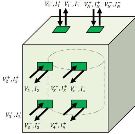
Fig. 1: A model transformer as an  $N$ -port network
