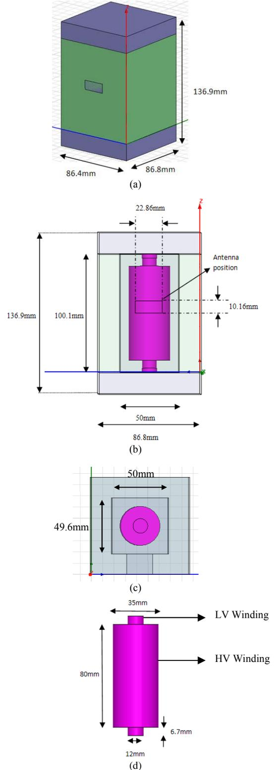
Fig. 2: Simplified model of transformer a) Three dimensional view, b) Side view of transformer model, c) Top view of transformer model and d) Side view of winding model
