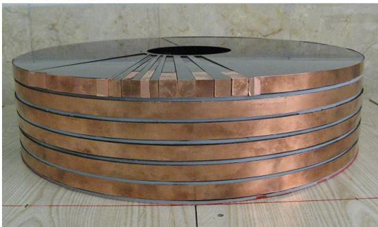
Fig. 1: Transformer winding model
