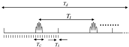
Fig.6: Timing of the pulses received in the receiver.
