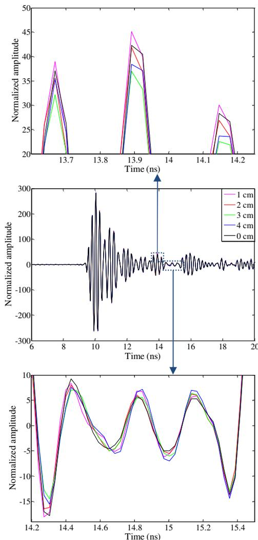
Fig.10: Reflected pulse for different length of radial deformation for 4cm<sup>2</sup> sector.
