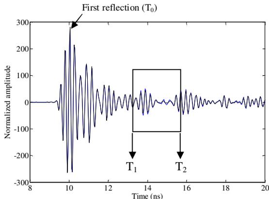
Fig.8: Received pulse can be windowed for detection of winding reflections
