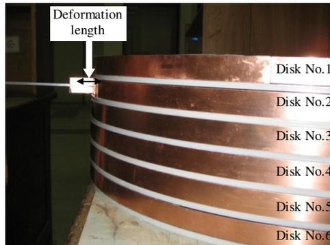
Fig. 2: Modelling of radial deformation (in disk No.2) and disk numbering
