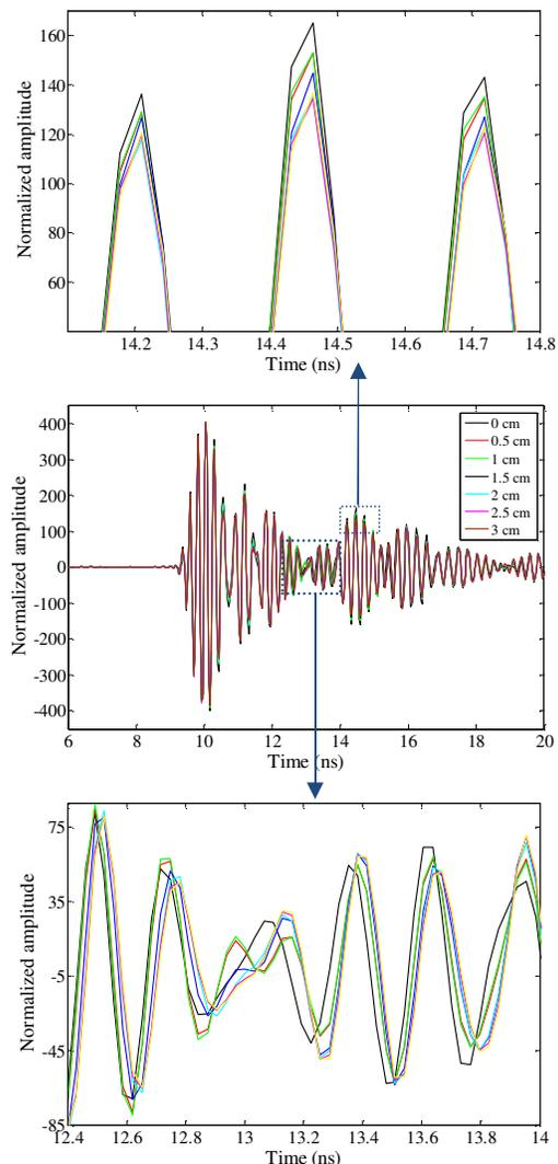
Fig.9: Reflected pulse for different axial displacement measurements
