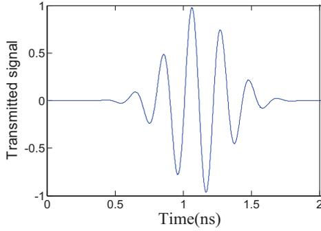
FIGURE 2. Transmitted UWB pulse.
