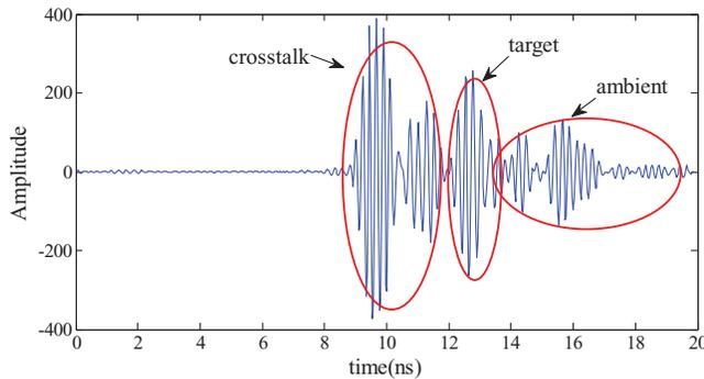
FIGURE 3. Different parts of a sample scan.
