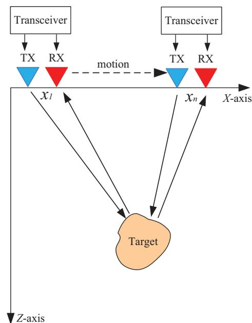
**FIGURE 1.** Data measuring process using UWB radar imaging.
