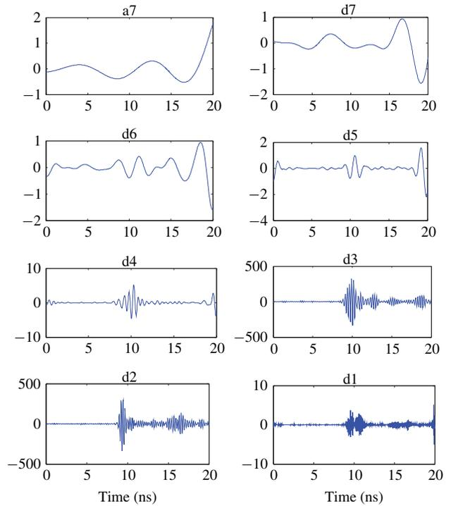
Fig. 16. Typical waveform of detail and approximate components of received signal for daubechies 16.
