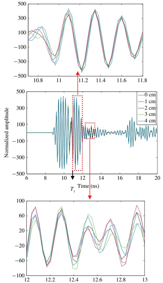
Fig. 11. Received pulse can be windowed to detect winding reflections.
