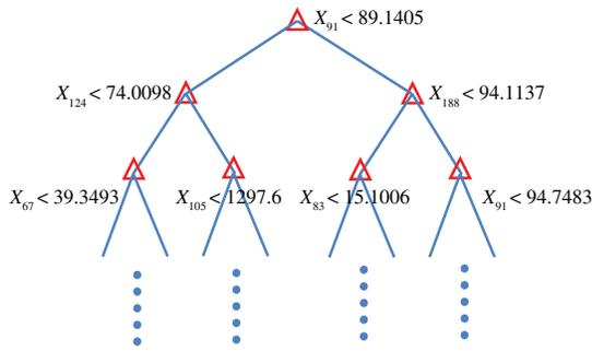
Fig. 19. Regression tree for estimation of radial deformation extent.
