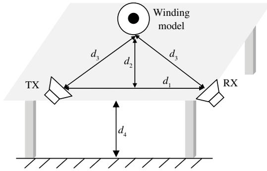
Fig. 6. Winding model in front of transmitting and receiving antennas.
