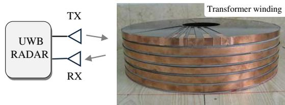
Fig. 1. Basic principle of monitoring by using UWB radar sensor.
