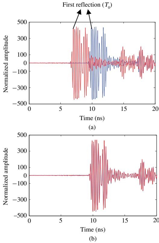
Fig. 10. Two received pulses (a) before and (b) after synchronization.
