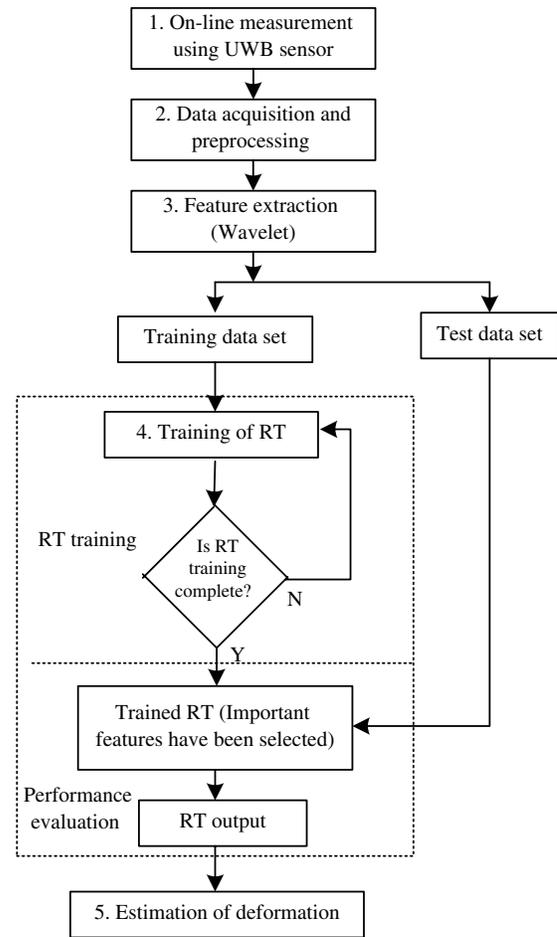
Fig. 20. Algorithm for estimation of radial deformation extent.
