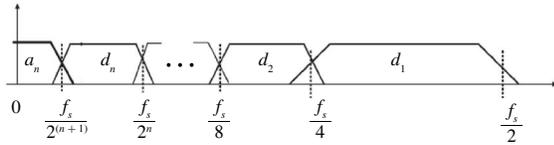
Fig. 15. Frequency ranges cover for details and final approximation.
