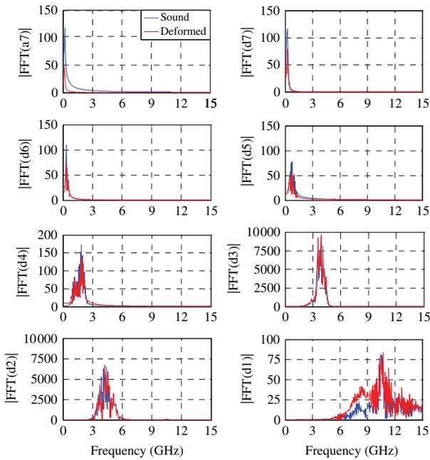
Fig. 17. Magnitude of FFT of details and approximation of two different received signal.
