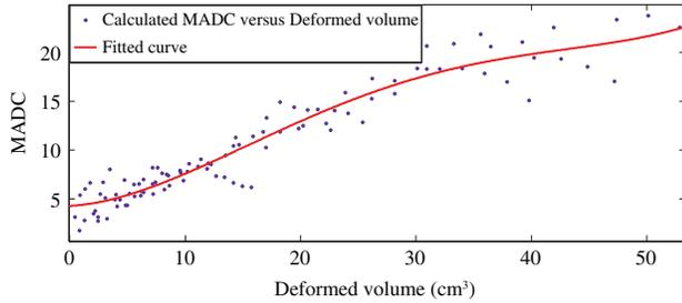
Fig. 14. Calculated  $MADC$  for second window versus deformed volume ( $\text{cm}^3$ ).
