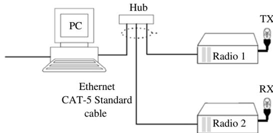
Fig. 3. Connection diagram of measurement set-up.
