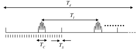
Fig. 9. Timing of pulses received in receiver.
