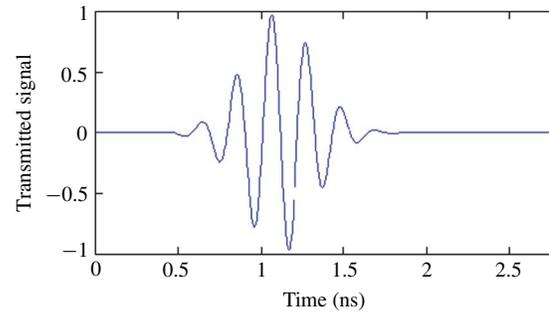
Fig. 8. Typical transmitted pulse.
