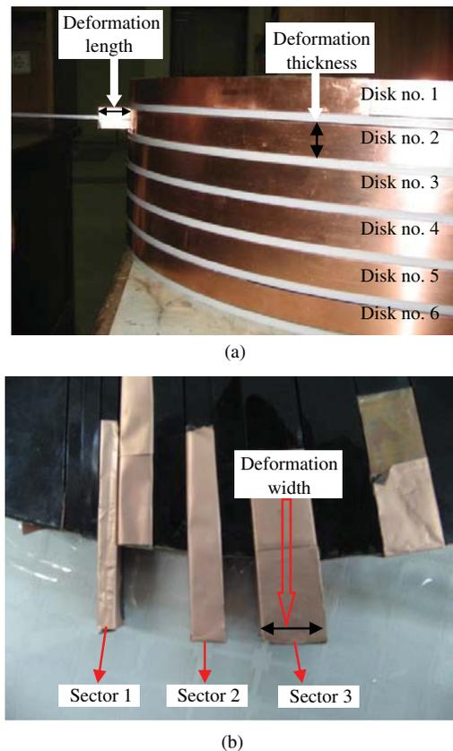
Fig. 2. Modeling of radial deformation. (a) Disk numbering and deformation length and thickness. (b) Deformation width.
